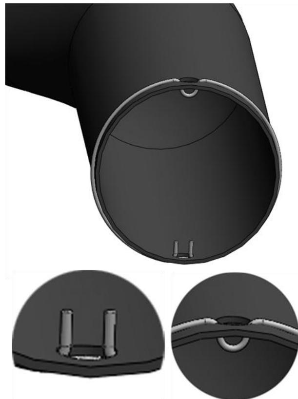
10. With the holes and bead rings installed in both pipes you can now install the silicone boots and then the positive air shutoff valve.
