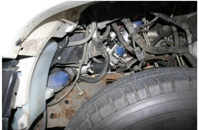
15. Reinstall wheel well/fender liner.
