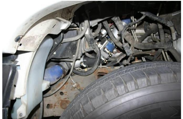
15. Reinstall wheel well/fender liner.
